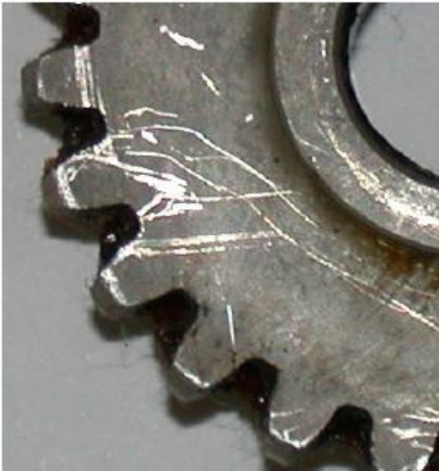
Unacceptable: Violation of surface treatment
