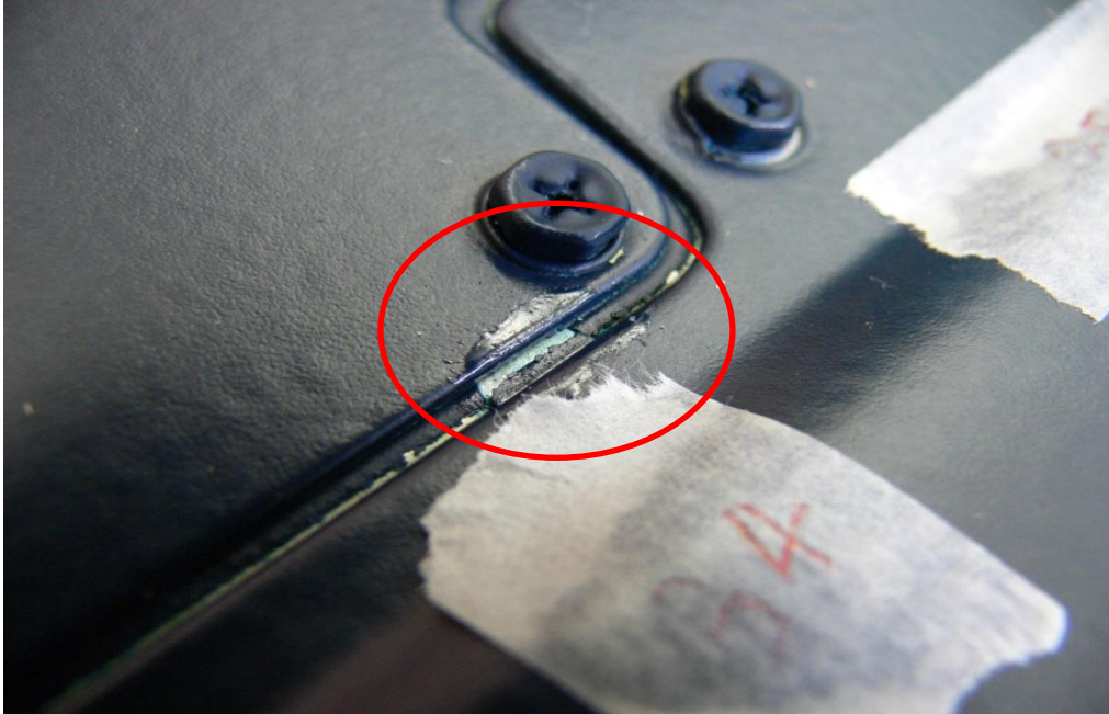
Touch up needed if damage exceed 1/2" in length
